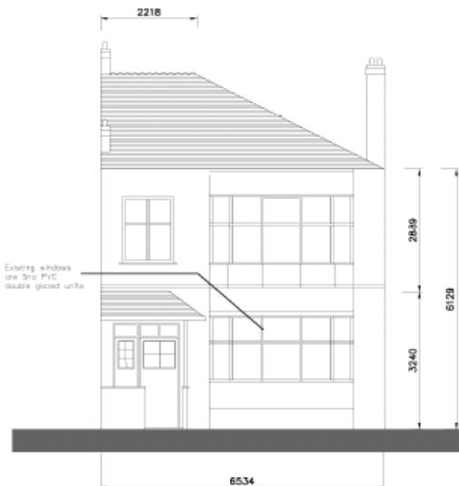
Existing Front Elevation
